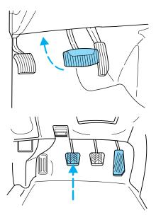
• Depress the clutch pedal (if equipped).
